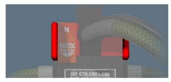
When the red grips are pressed together, the harness inflates. When the red grips are released, the harness deflates.
