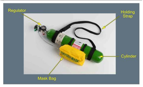
The portable oxygen bottle - or cylinder - with a mask attached supplies first aid oxygen to passengers or cabin crewmembers. The crewmembers can select an oxygen flow rate of 2 Liters Per Minute(LPM) or 4 LPM.
